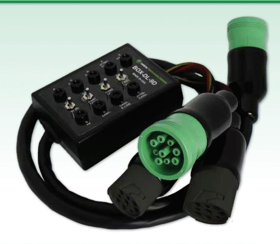
If you work on J1939 9-pin Deutsch based vehicle systems, you will have to have one of these in your toolbox, or two! The J1939 Breakout Box allows multiple tools to be connected to a vehicles data buses to support vehicle integration testing, logging, or debugging. It is extremely useful in troubleshooting connection and or messaging problems.
